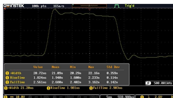
Waveform of a 35V 20ns pulse
